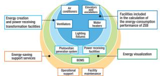
\* BEMS (Building Energy Management System): A system that visualizes and centrally manages the energy usage of an entire building.
